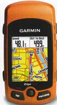
IBIKE AERO (OR ANOTHER ANT+ POWER METER) TO GARMIN EDGE 705 BENEFIT: Power readings on Garmin screen and in related software DRAWBACK: Slight lag in on-screen power reading
